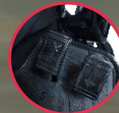
HYDROSTATIC TRANSMISSION WITH TWIN HST PEDAL
