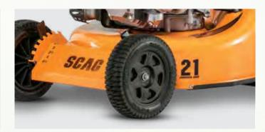
Strong, stamped steel deck ensures years of worry-free performance and a consistent cut. Replaceable side wear protection.
