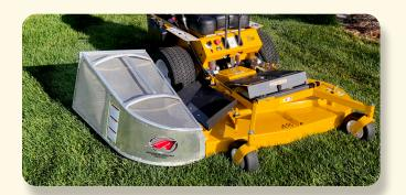
The Accelerator® grass catcher can be placed on any Model R side discharge deck and used for collection of yard debris, leaves, and grass clippings.
