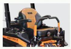
Torsion-spring suspension seat adjusts to operator's weight to provide superior comfort on most models, excluding 31FX and 36BV. All seats feature 4-point rubber iso-mounting to further absorb vibration.
