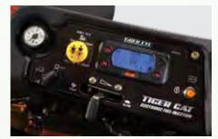
Operator-friendly instrument panel includes a conveniently located ignition switch, cutter-deck-engagement switch, choke, throttle controls and Tiger Eye™ Advanced Monitoring System.
