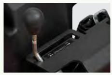
Dual, integrated ZT-5400® Hydro-Gear® transaxles give you responsive, dependable power. A cooling fan on each unit keeps operating temperatures low. Two-speed settings let you choose either Low Range to travel up to 12 mph or High Range for up to 16 mph.
