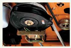
Ogura GT2 (108 ft lb) PTO clutch brake for easy deck engagement. Adjustable internal air gap for long life.
