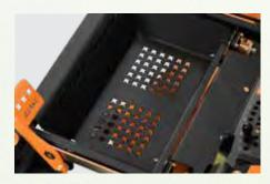
Pierced, extruded-steel footplate is rubber iso-mounted for enhanced comfort.
