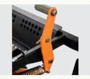
Cutter-deck-lift foot pedal is spring-assisted and makes raising the cutter deck smooth and easy.
