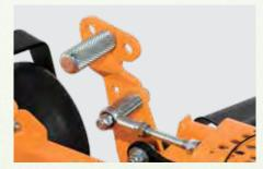
Adjustable, 3-position deck-lift foot pedal makes changing the height-of-cut fast and easy. Adjusts from 1" to 5" in ¼" increments.
