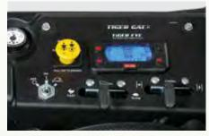
Operator-friendly instrument panel includes the Tiger Eye™ Advanced Monitoring System, which keeps a constant, real-time "eye" on important system functions of the Tiger Cat II. (Specific functions vary by mower model and engine.)
