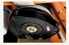
Heavy-duty Ogura GT3.5 clutch features 250 ft lb of holding strength. Adjustable air gap for long life.
