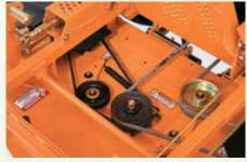
Entire foot plate area lifts to provide complete access to the top of the deck for easy servicing.
