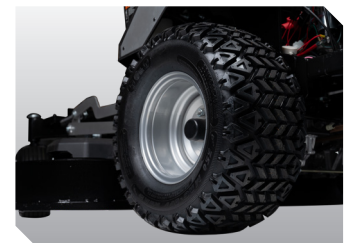
More Traction – Large 22" rear tires with semi-aggressive tread pattern
