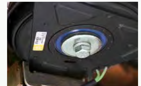
Dependable Ogura clutch engages and disengages the blades quickly and easily. Adjustable air gap for long life.
