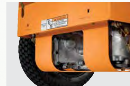
Dual hydraulic ZT-2800® transaxles with cooling fans and steel fan covers allow independent, amazingly smooth and positive power to each wheel; two independent units with charge pumps and all-metal gears. Rear skid plate protects the underside and transaxles from impact damage.
