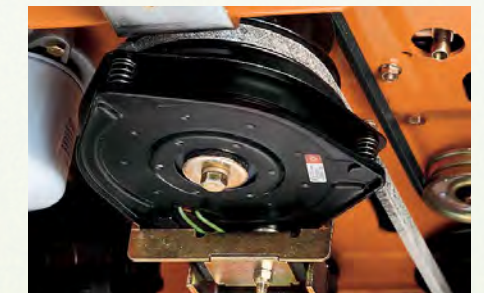
Ogura GT1 (74 lb) PTO clutch brake for easy deck engagement. Adjustable internal air gap for long life.
