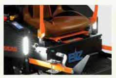
Standard LED lights illuminate the way to and from the garage or trailer in low-light conditions.
