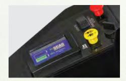
Full-featured display screen shows battery charge level, hours of run time and provides system diagnostics.
