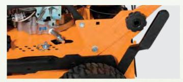
Single-point, rider-style height-of-cut adjustment. Cutting heights from 1½" to 5" in ¼" increments. Pin installs from the top for quick, easy changes.
