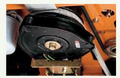
Ogura GT1 (74 ft lb) PTO clutch brake for easy deck engagement. Adjustable internal air gap for long life.
