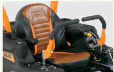
Comfortable, thick-cushioned seat is easily adjustable and delivers a high level of operator comfort. Shock-absorbing action added with 4-point iso-mounting.
